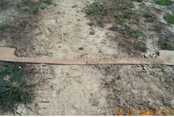
Figure 12 – damage on board 1, topsoil lane
