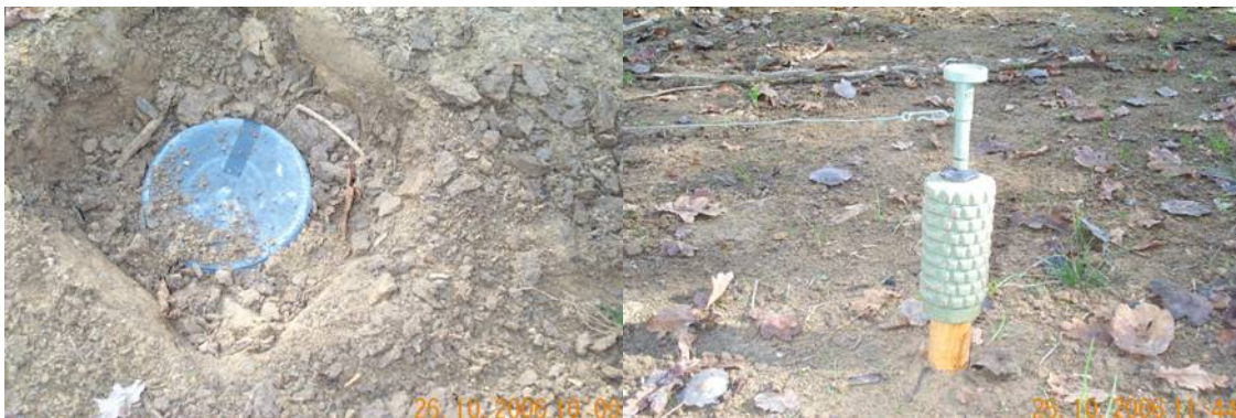
Figure 8 – AP mines PMA-3 and PMR-2A prepared for testing of “MINI MINE WOLF“
