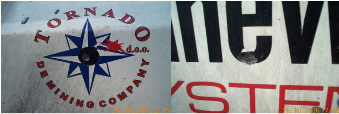
Figure 9 – Shrapnel marks of PMR-2A on “MINI MINE WOLF“
