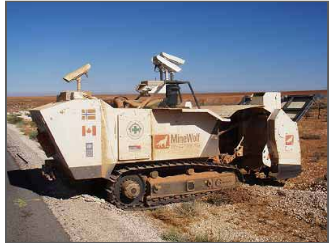
2 nd Mini MineWolf in operations in Jordan with remote video guidance system
