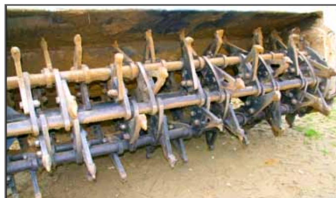
Post-detonation results: the MineWolf tiller suffered virtually no damage
