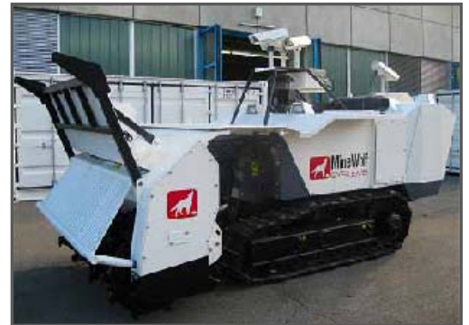
Mini MineWolf remote-controlled demining machine equipped with remote video guidance system
