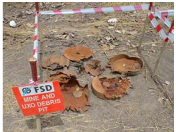
Examples of AT mines destroyed by MineWolf during operations
