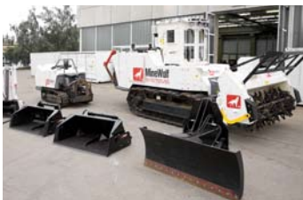
MineWolf and Mini MineWolf with a range of attachments
