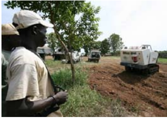
Operator handling the Mini MineWolf remote controlled
