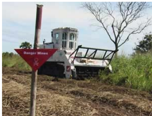
MineWolf, a mechanical mine-clearance machine, working in Yei, South Sudan. All photos courtesy of MineWolf Systems
